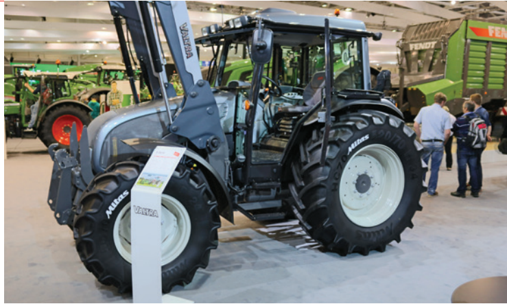
An A Series Valtra tractor mounted on Mitas tires HC70 520/70R34 (rear) and HC70 420/70R24 (front).
