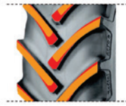
Conventional profile design AC 70G Tread pattern
